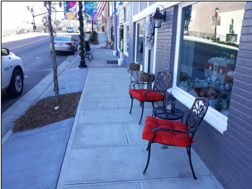
56 – Middle St from Valley to Main Updated sidewalks but need to enforce merchant's products to maintain 4' clear width
